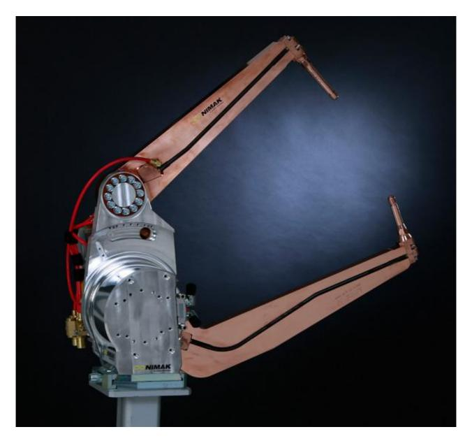
Nimak offers the galaxyGun for resistance welding of mixed materials, conventional steel, and aluminum. The gun opens and closes quickly, and its electrode arms open wider than previous products, the company reports, to prevent interference contours.
