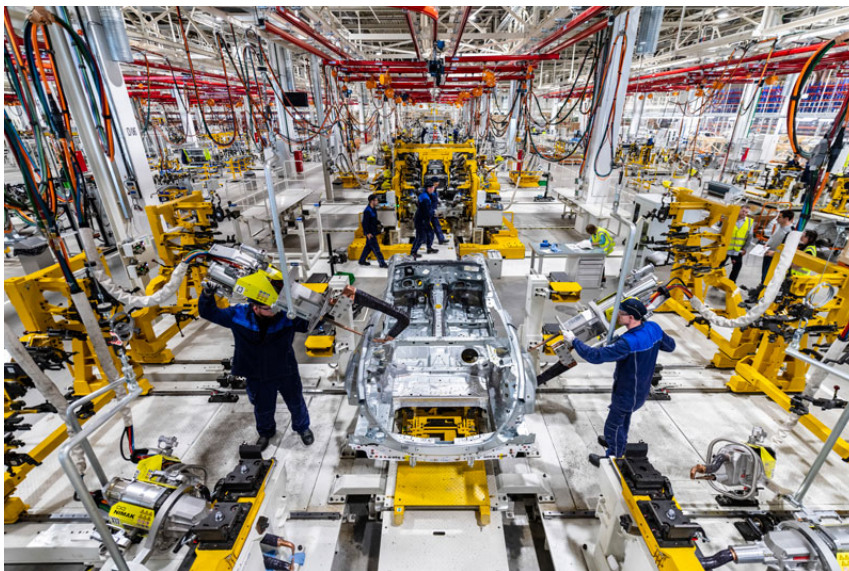
Image 1: NIMAK manual welding guns in production at the new Mercedes-Benz assembly plant in Russia.
